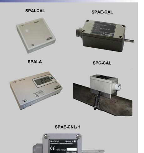
These probes allow to measure the ambient temperature in a room and provide a 4-20 mA loop powered output signal. The measure element (Pt 100 platinum RTD probe) used ensures an excellent repeatability of the measures.
